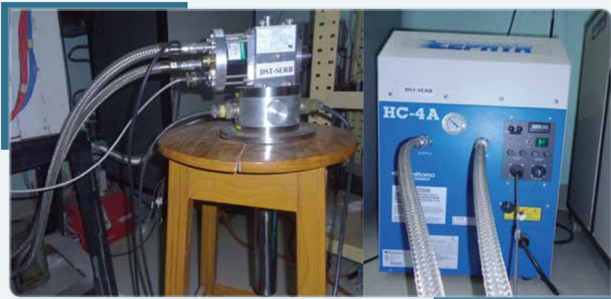
Fig. 3.23: Close cycle refrigerator with compressor procured from the project
